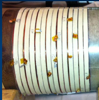
BSCCO-2212 Cable - Transport measurements show that FNAL cable attains 105% J_c of that of the single-strand
