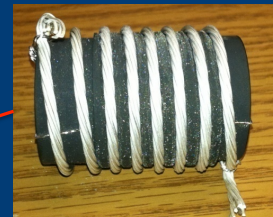
Multi-strand cable utilizing chemically compatible alloy and oxide layer to minimize cracks
