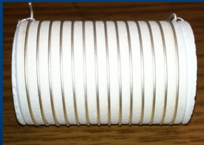
BSCCO-2212 Cable - Transport measurements show that FNAL cable attains 105% J_c of that of the single-strand
