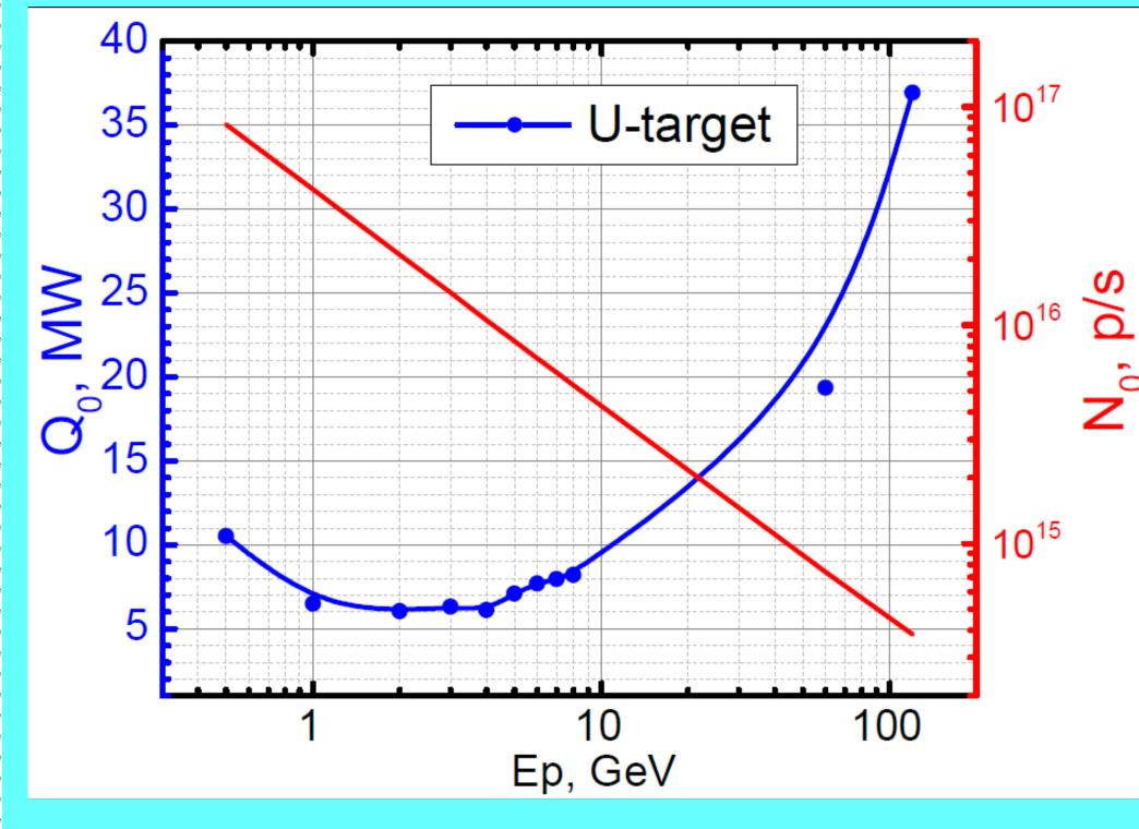
$3.10^{15}$  p/s at 120 GeV. The same plot gives the proton beam power necessary to equate the consumed and released energies  $(Q_0)$ , it has a minimum of  $\sim 6$  MW in the range 2-4 GeV. In these calculations the power to tween the energy released in the target to the proton frun the accelerator in the idle mode was assumed to be
