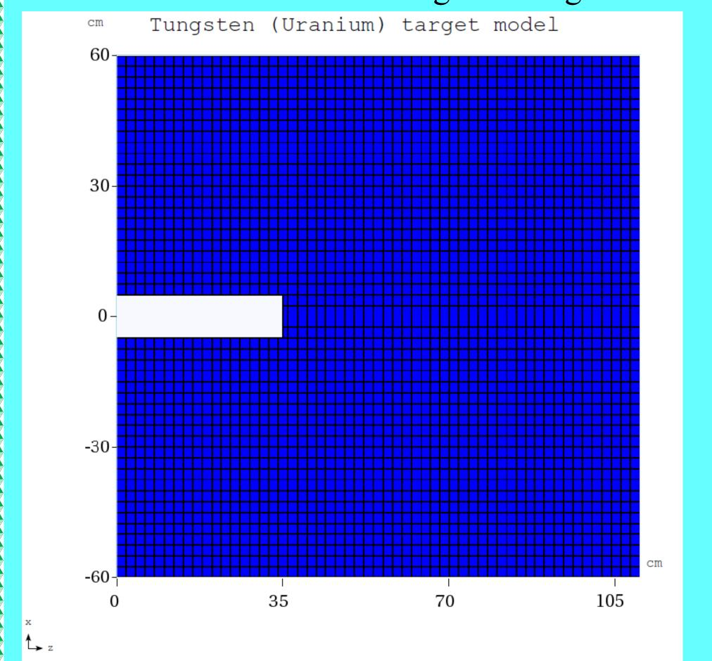
sion were chosen to minimize the neutron leakage from the surface down to the level of <2%. There is a 10 cm in diameter 35 cm beam entrance hole at gible). the target center. The Figure below shows the neutron production in the target as a function of the proton beam energy.
