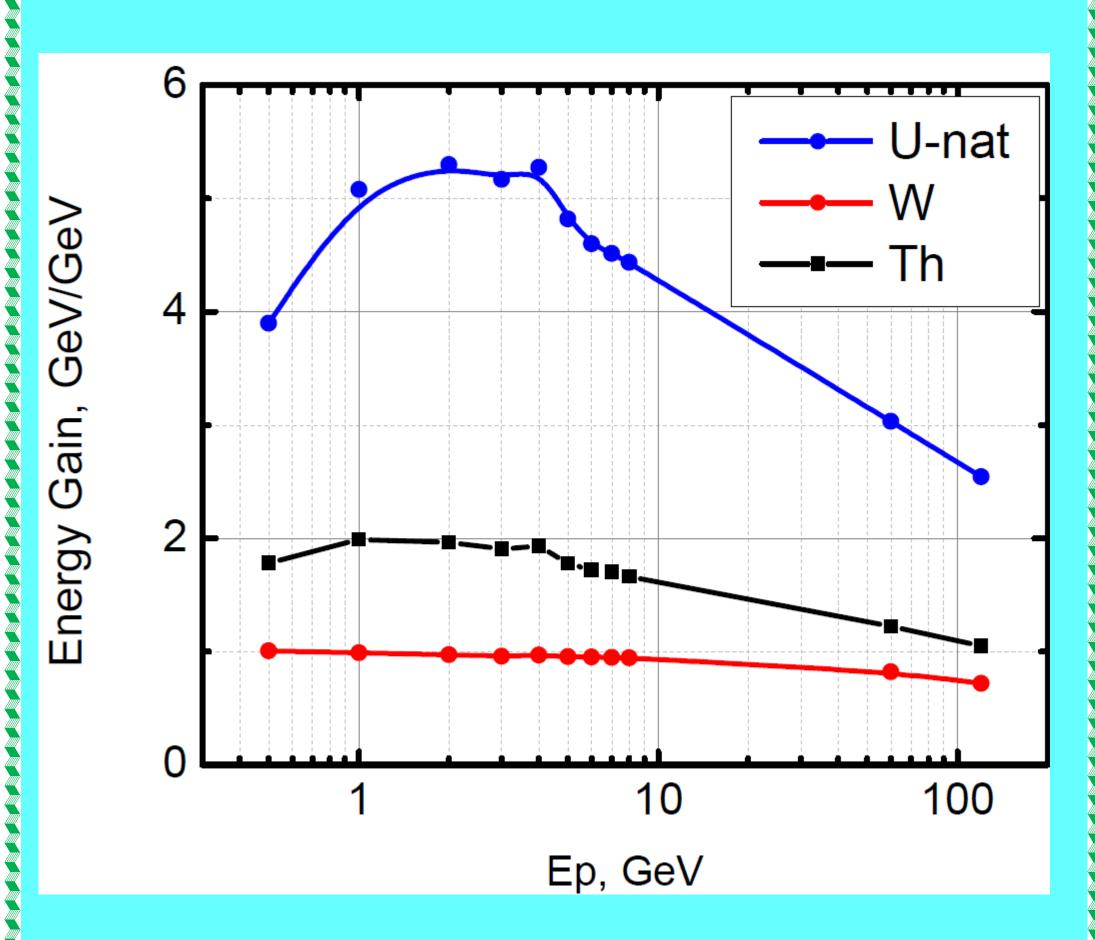
and the peak energy gain in the  $^{nat}U$  is  $\sim 5$ . The Th target reveals the peak gain  $\sim$ 2, while there is no gain in the W target (as the fission cross section of W is negli-
