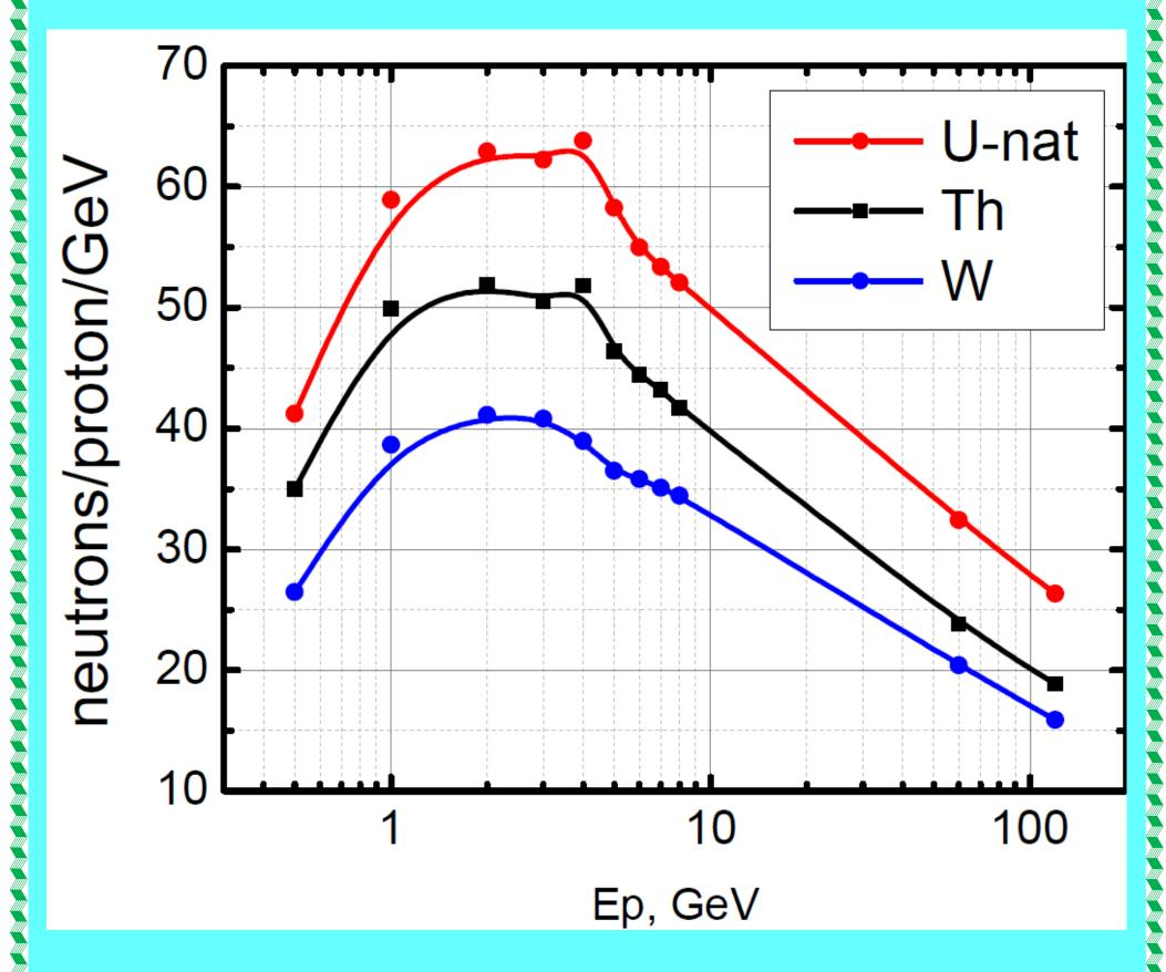
The peak neutron production is between 1 and 4 GeV, it is 50% higher in natU than in W and 20% than in Th targets. The energy gain (or the ratio be-
