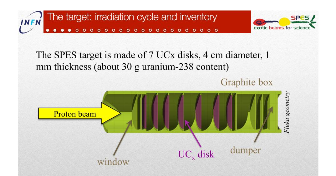
The irradiation cycle lasts <u>14 days</u>, a total of <u>10<sup>21</sup> protons on</u> <u>target</u> and a total of <u>10<sup>19</sup> fissions</u> are induced on the target
