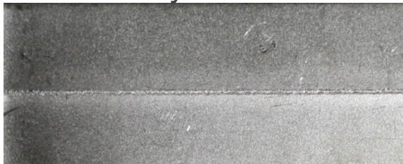
Keyhole weld root side cavity exterior
