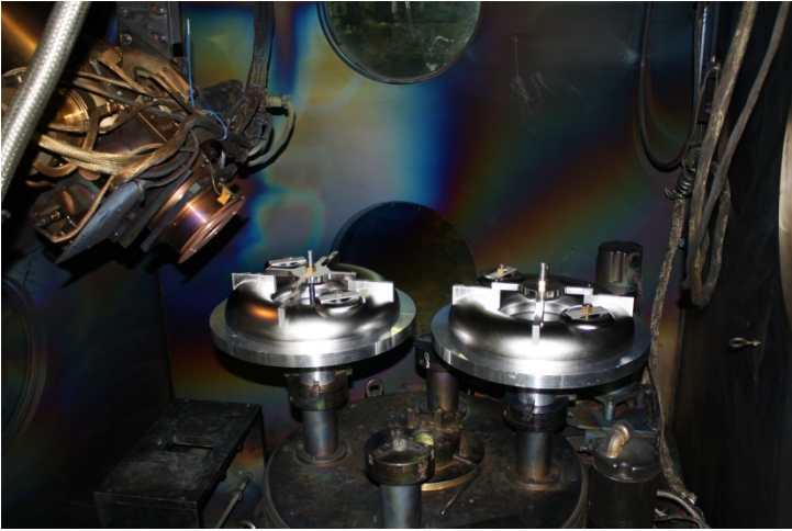
Setup for welding gussets
