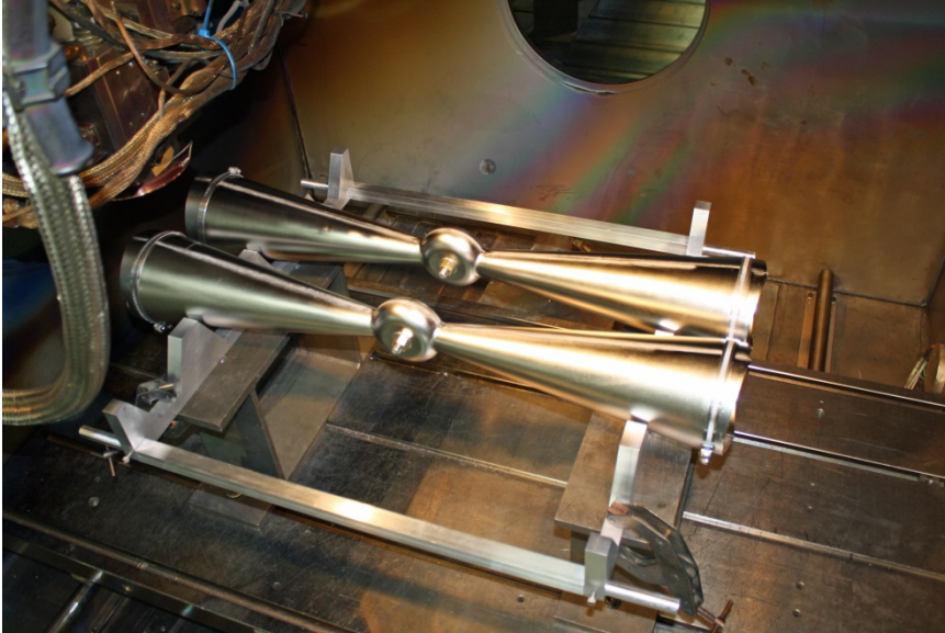
Center Conductor seam weld setup
