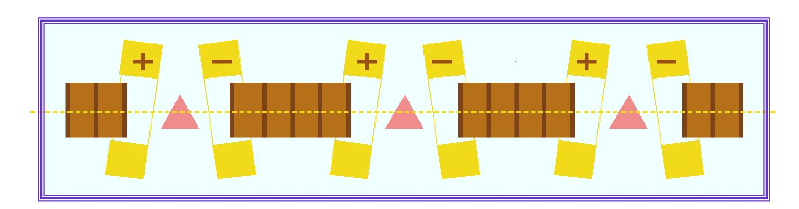
The transformation is achieved by alternating inclination of solenoids at small angle (typically 10-40 mrad) in horizontal plane. It gives rise to transverse periodic orbit and dispersion which can be used for emittance exchange with help of wedge absorbers. Such a channel has about the same performance as other known 6D cooling channels with a comparable field being simpler in construction.
