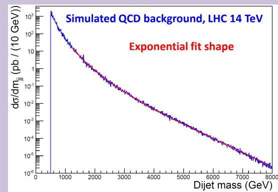
Flat K-factor of 1.40 No pile-up No EW Sudakov Minimal detector smearing Dijet trigger left free
