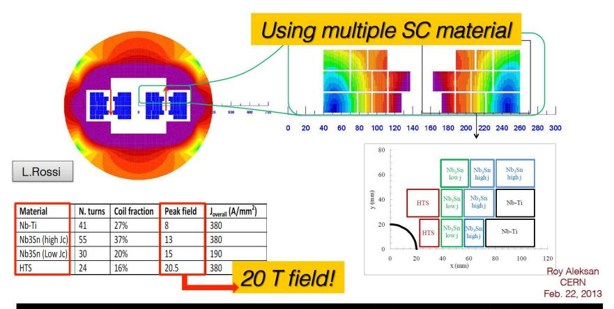
Magnet design: 40 mm bore (depends on injection energy: > 1 Tev) Approximately 2.5 times more SC than LHC: 3000 tonnes! (~4000 long magnets) Multiple powering in the same magnet for FQ (and more sectioning for energy) Only a first attempt: cost and other shapes needs to be also investigated
