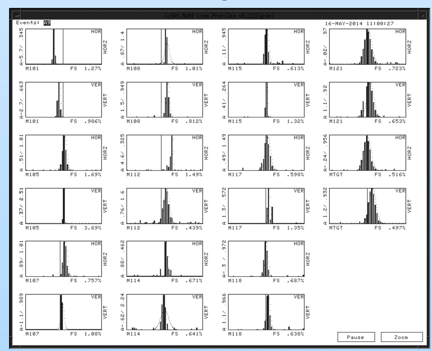
**SEM Gain Stability** for a Ti foil [1] target detector exposed to **1.43 x 10<sup>21</sup>** protons and a Ti wire detector currently exposed to 1.74 x 10<sup>20</sup> protons. The foil SEM grid was replaced by wires to achieve significantly less residual activity.
