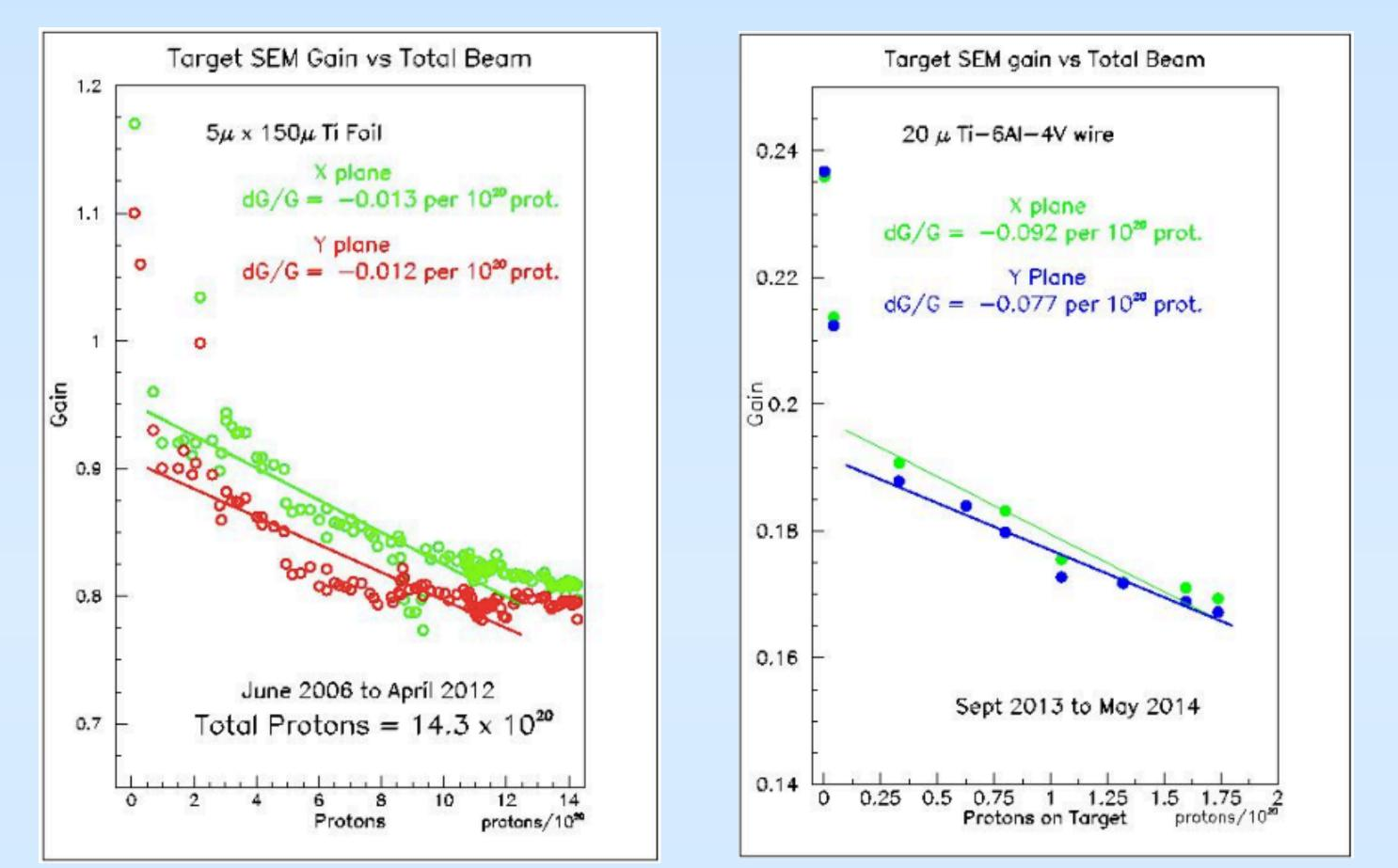
\*Ti Grade 5 high performance alloy which contains 6% AI and 4% V. It was selected because it can be manufactured to smaller wire diameters.
