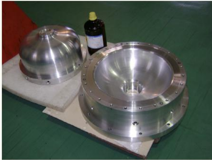
Half cell forming die & Punch set
