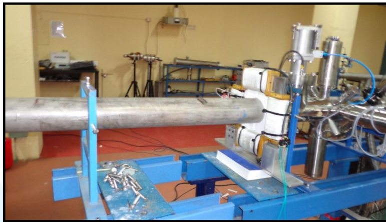
Dipole corrector magnet assembly installed in FOTIA beam line
