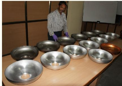
Formed Half cell – Alu, Cu, Nb
