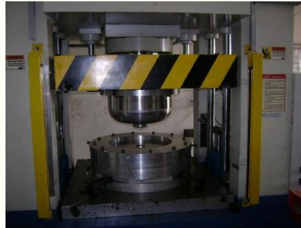
Die-Punch set mounted on the press
