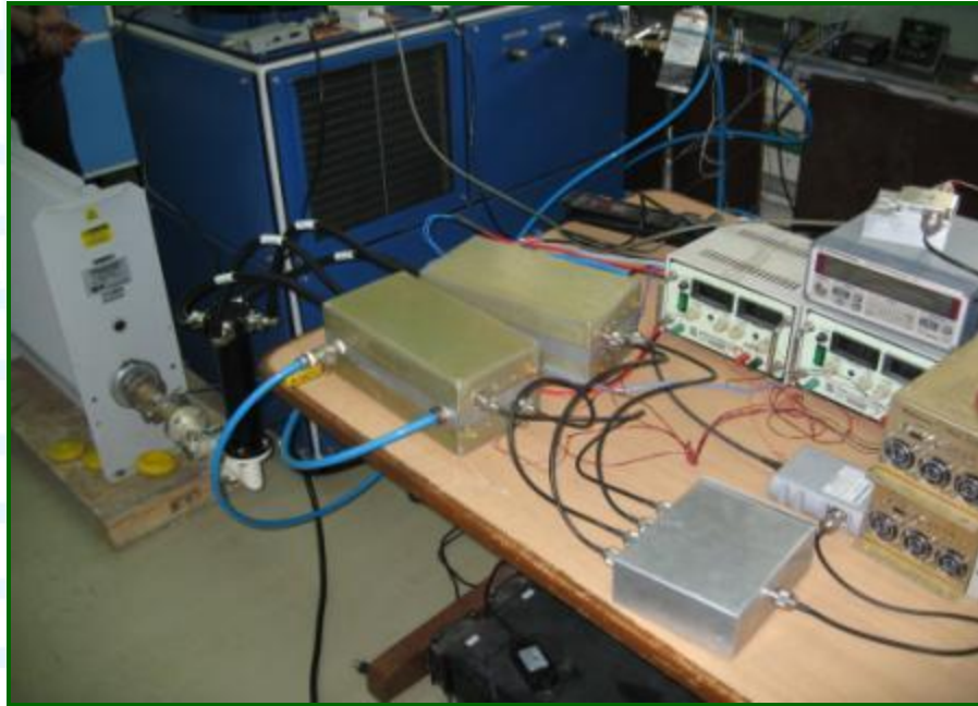
Prototype testing of 3 kW RF amplifier
