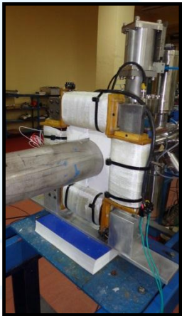
Dipole corrector magnet assembly installed in FOTIA beam line
