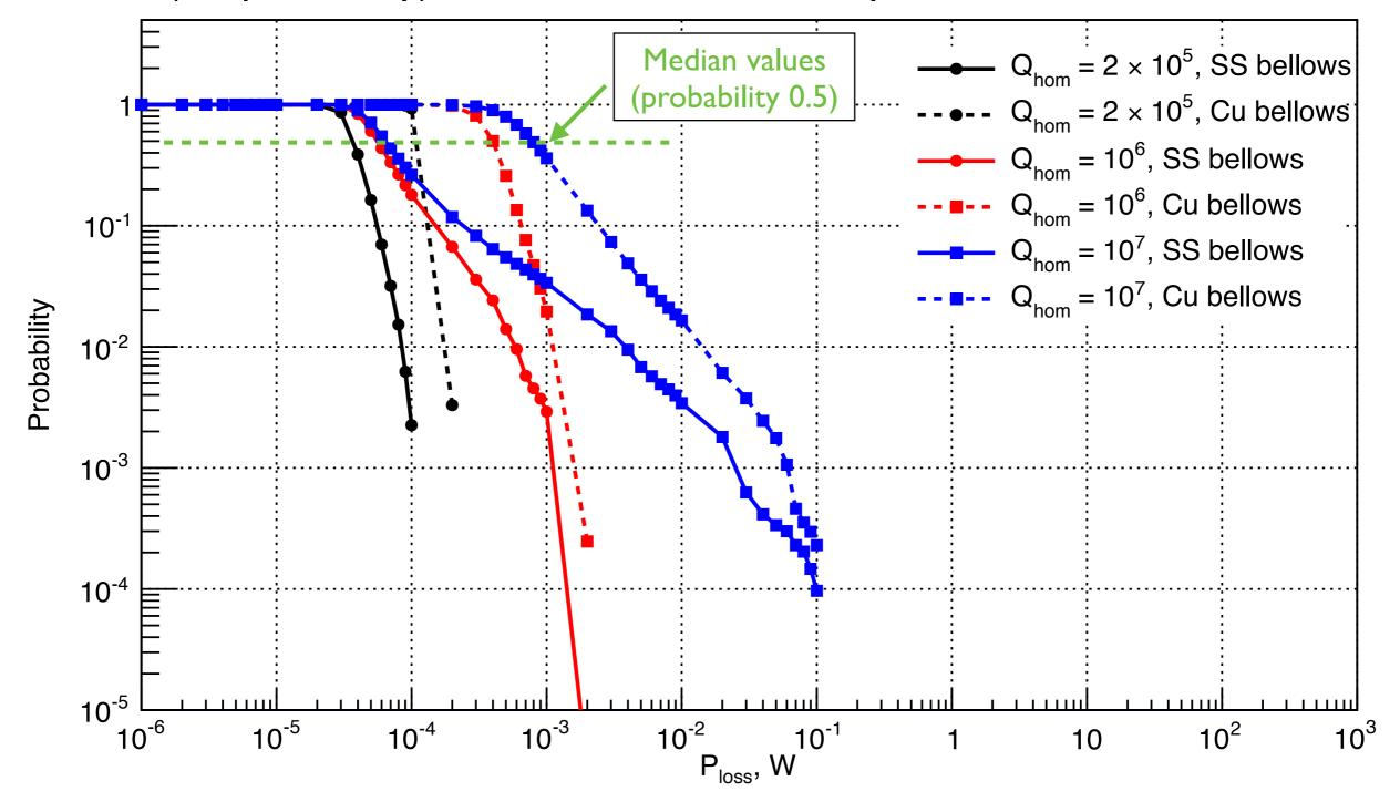
Heat load at 2K due to resonance HOM excitation is not a problem
