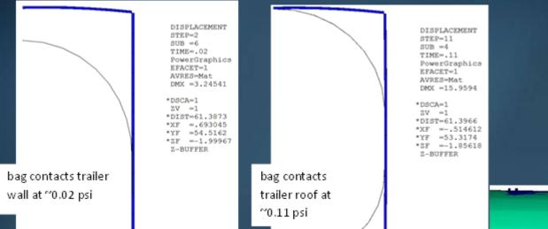
Pressures calculated using finite element analysis are consistent observations. The maximum membrane stress calculated was 640 psi.
