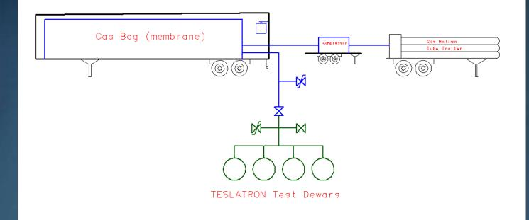
Gas bag mounted in a insulated rented trailer with an electric heater to keep gas bag pliable during the winter
