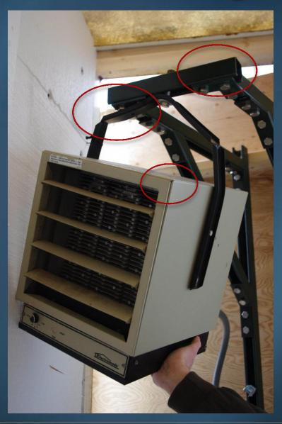
Force of bag on heater bent the top heater bracket. Bracket was constrained by bolts on the Unistrut<sup>®</sup>. Resulted in the top-right corner facing more forward
