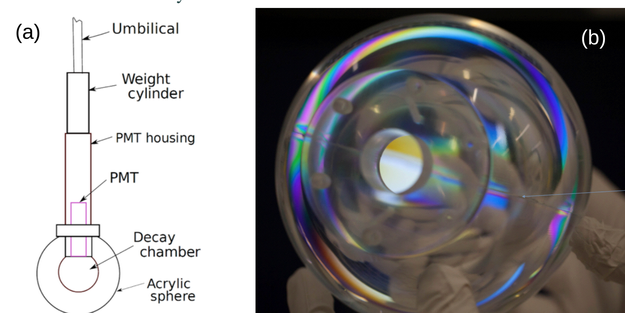
Figure 5: The Cherenkov source design (a) and a prototype acrylic sphere (b).
