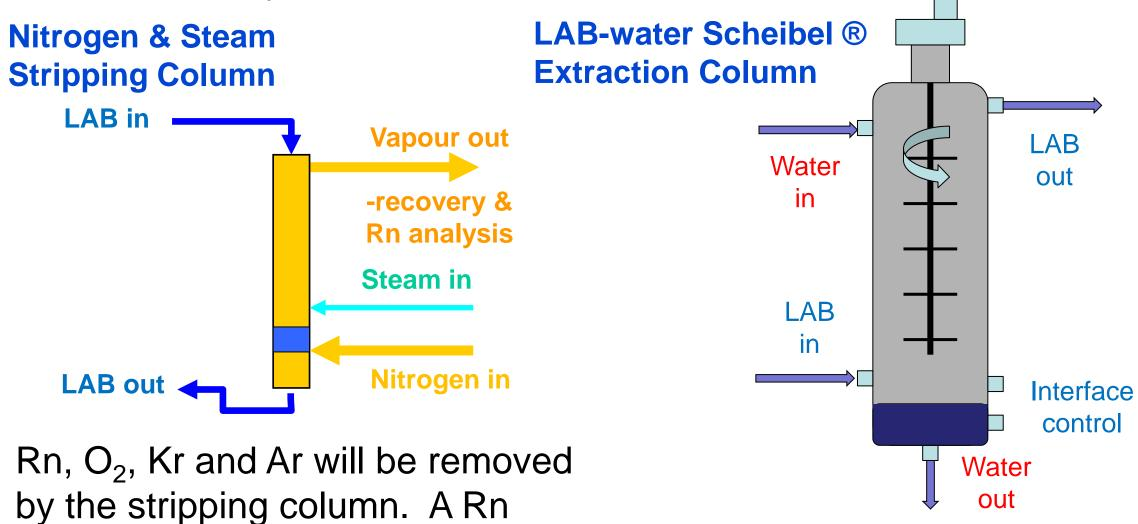
This 150 L/min process has been for use with this column (using cryo shown to remove <sup>40</sup>K and Ra and is also effective for removing recoil <sup>210</sup>Pb techniques) and efficiency tests are (see ref. 2). It will be used in the solar neutrino & double beta decay phases.
