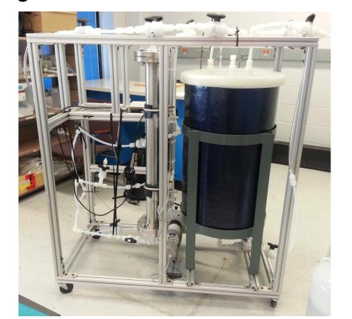
This 15 L/min distillation, performed as the LAB is moved underground, improves the optical path length and removes <sup>7</sup>Be, Pb, Th, U with > 90% efficiency.
