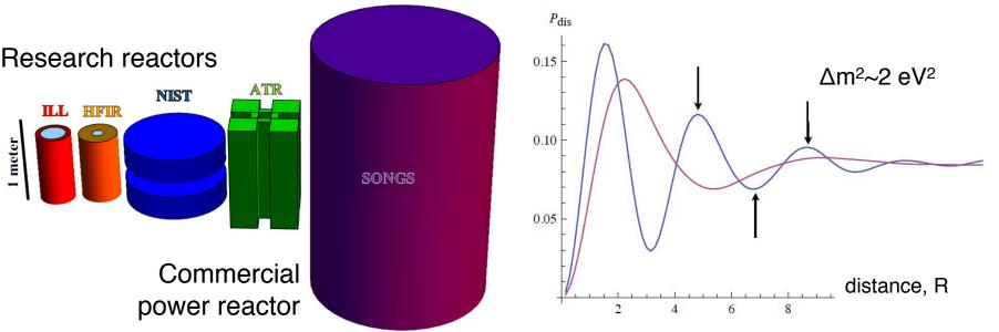
Research reactors have compact cores with diameters <1m
