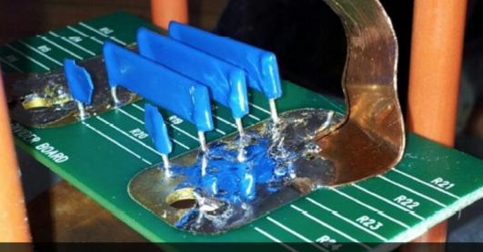
**Unprotected resistors** damaged after over-voltage
