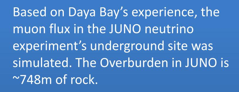
$\square$  Muon rate: 0.0030Hz/m<sup>2</sup>. ■ Average energy: ~215GeV.
