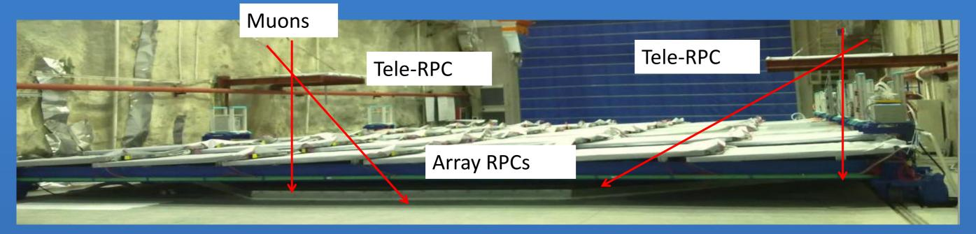
2 Telescope-RPC about 2m above bottom array RPC in each hall; Muon position resolution of RPC tracking system ~0.1m; The combined telescope-RPC and and array RPC system can measure the muon trajectory as shown below.
