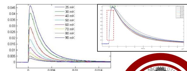
Pulse shapes of photon detector
