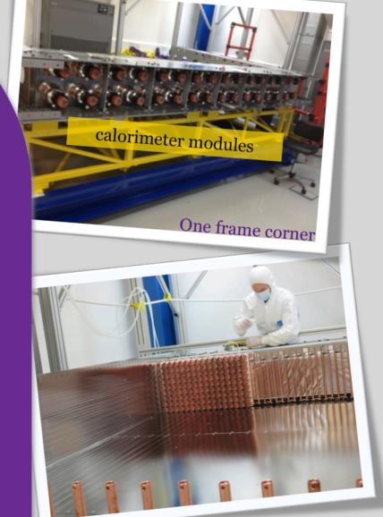
The tracking detector is being assembled in quarters, at UCL's Mullard Space Science Laboratory. The frame of the first quarter is complete and the calorimeter modules, consisting of PMTs coupled to blocks of plastic scintillator, have been integrated around the edge. The gastightness of the frame has been tested, and the first tests of the gas system and radon emanation technology have been performed.
