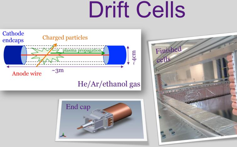
The tracking in the Demonstrator Module is performed by 2034 drift cells operating in Geiger mode. A central anode wire is surrounded by twelve cathode wires, in a helium-argon gas mixture. The passage of a charged particle ionises the gas, resulting in an electron avalanche. This produces a plasma that propagates along the anode wire. The time difference between the signal arriving at each end provides the longitudinal location of the charged particle. (See also the poster by F. Nova.)
