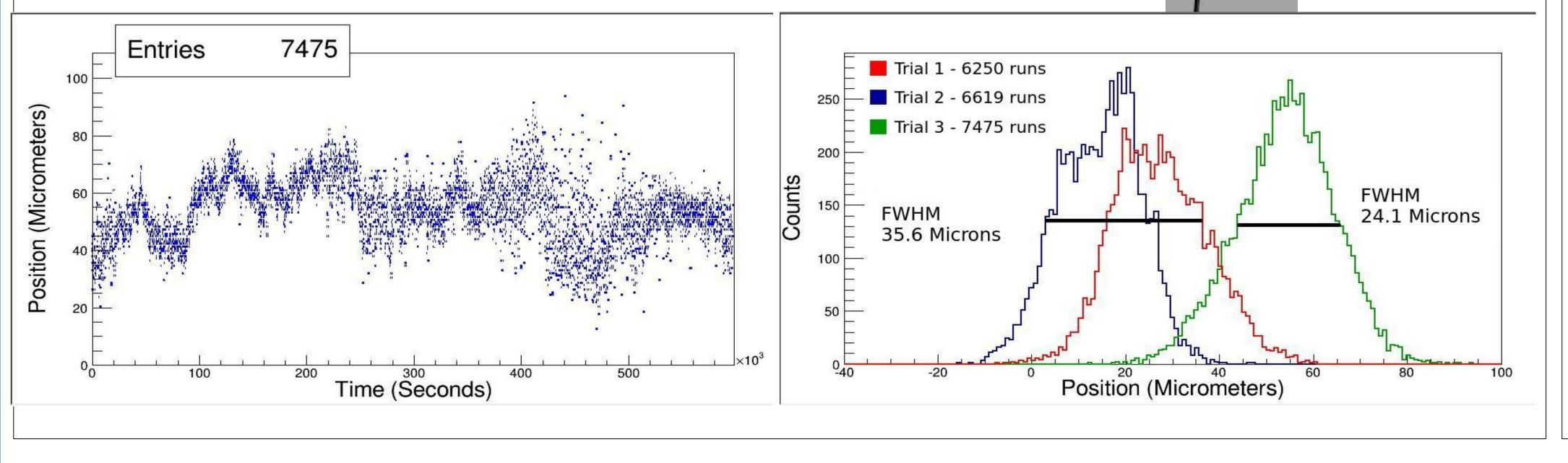
Above, LED peak positions in the reference block compared with lab Shown temperatures over time. right, relative fluctuations in same LED peaks relative versus There is temperature fluctuations. high negative correlation, denoted by the Pearson coefficient, between individual LED peak and the temperature but not between the predicted <sup>207</sup>Bi peak values and temperature. This was proven true for any measured source peak as well.
