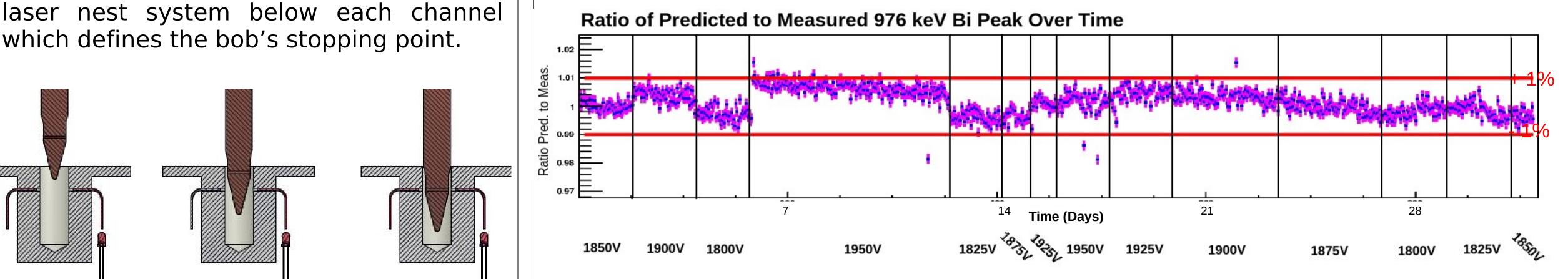
The discontinuities in the data correspond to changes in HV on the 8-inch PMT which mock possible operational jumps. Even with these perturbations the system holds up
