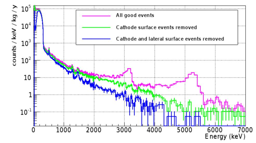
This leads to a background rate of approximately 1 count/keV/kg/y in the region of interest around 2814 keV, given per unit mass of detector material (CdZnTe), and the
