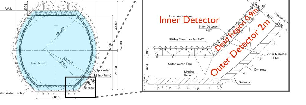
99,000 20" PMTs for ID (20% photo-coverage) and 25,000 8" PMTs for OD (same as SK) are installed. The PMTs are supported with stainless-steel frames.
