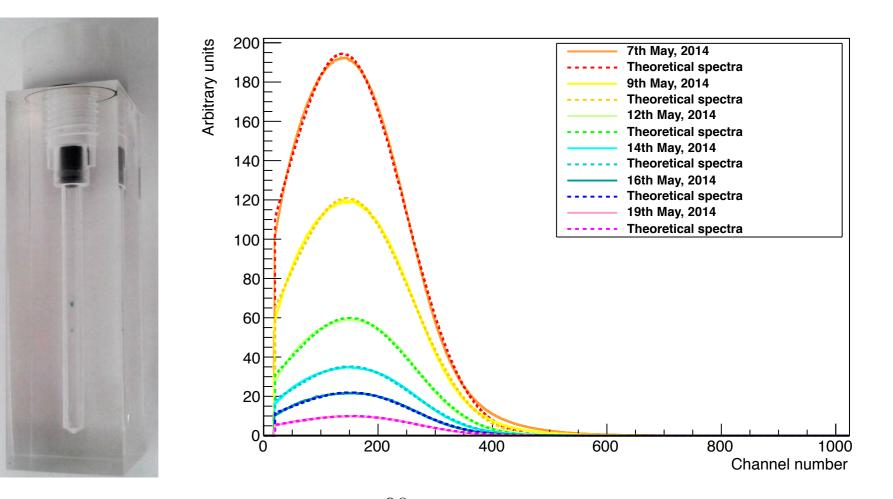
Measurements of a prototype  ${}^{90}$ Y filled capillary in a small desk-top setup at U. Sussex over a period of 2 weeks showing source decay. The measured scintillator energy deposit has been fitted to the theoretical  ${}^{90}$ Y  $\beta$  spectrum. The earliest measurement is thought to show the effects of event pileup.
