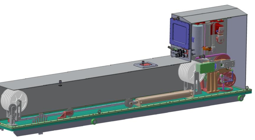
New URMs must be completely compatible with LAB. To avoid mine air getting into the detector, the URMs are sealed and filled with nitrogen gas. The source containment tubes (not shown) will be air-tight and closed with gate valves until connected to the Universal Interface (see below).
