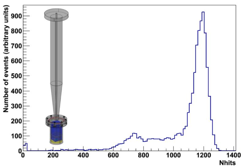
The gamma rays escape into the main SNO+ volume largely unimpeded, and the detector triggers on their sum energy, giving a calibration point near the endpoint energy of the  $^{130}$ Te decay. The electron tag creates a nearly background-free set of calibration data that may be used, for example, to study low statistics non-Gaussian tails in the detector resolution function.
