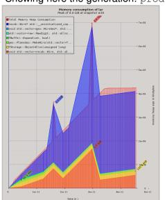
We can identify a transient peak up to 6.6 GiB and the code which allocated it (not shown:
