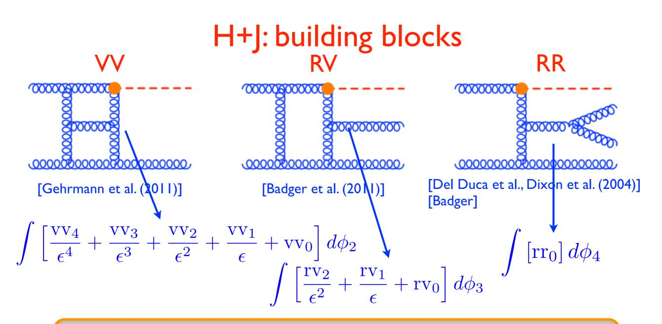
Problematic part is to extract implicit IR poles from RV and RR in a FULLY-DIFFERENTIAL way, i.e. without doing the PS integration
