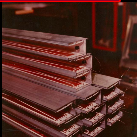
Install cathodes in extrusions
