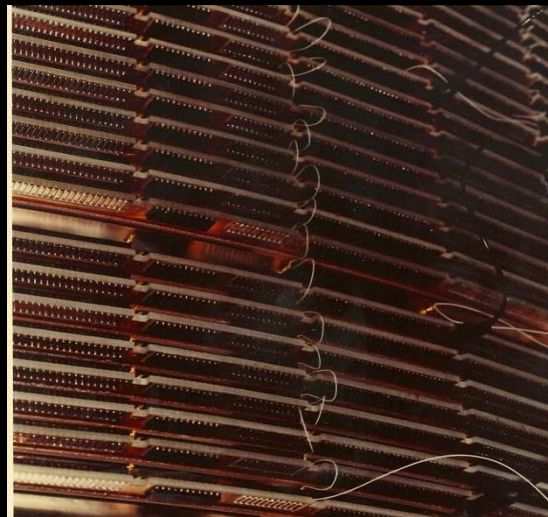
Traces to gang \eta\phi signals from a fixed depth segment.
