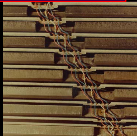
Can't weld to uranium. Supersonic Indium darts for HV connections
