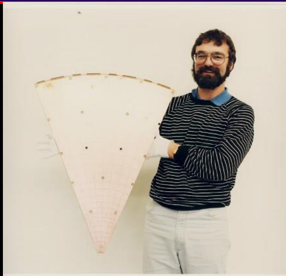
Rout signal board into \eta\phi pads
