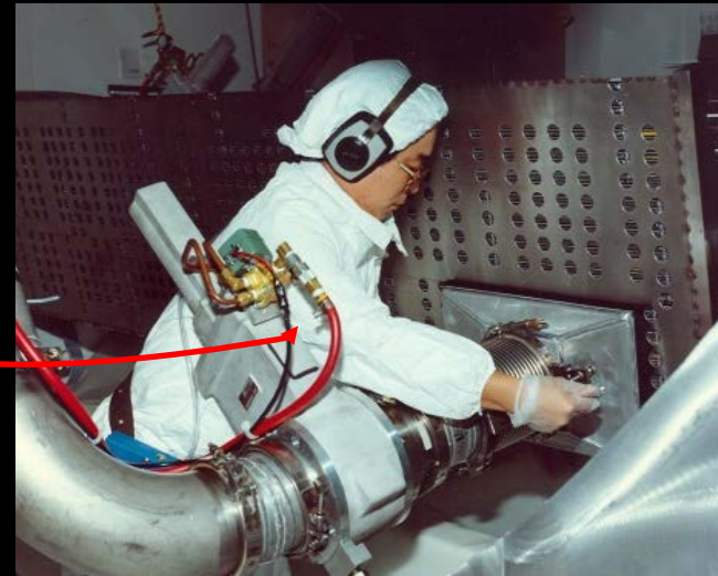
Last step: Power vacuuming; gate valve to evacuated tank made a huge sucking noise carrying out \text{UO}_2 dust
