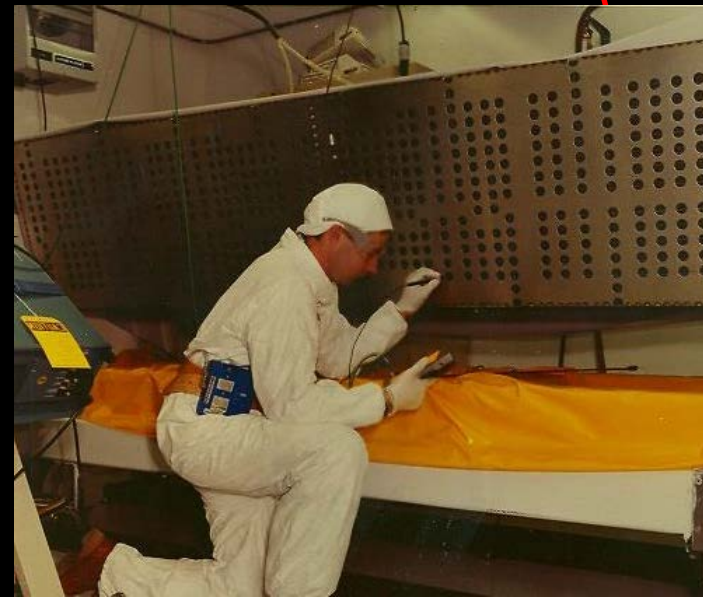
Probing CCFH module for defects after scrubbing
