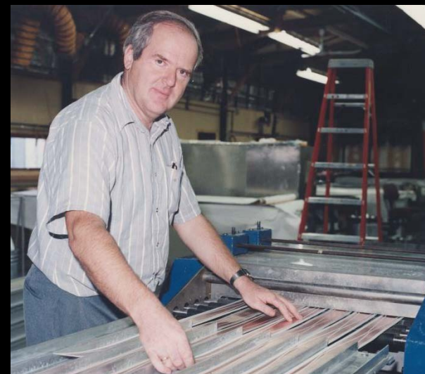
Routing PDT cathodes on Thermwood machine
