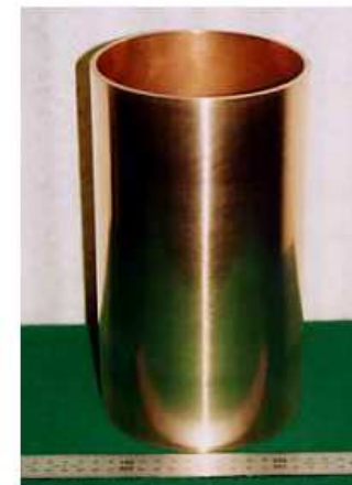
Figure 5: Cu/Nb/Cu clad seamless pipe made by cladding, hot&cold rolling, deep-drawing and spinning.
