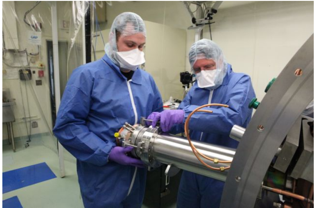
Coupler Assembly Leak Test Cavity Insertion
