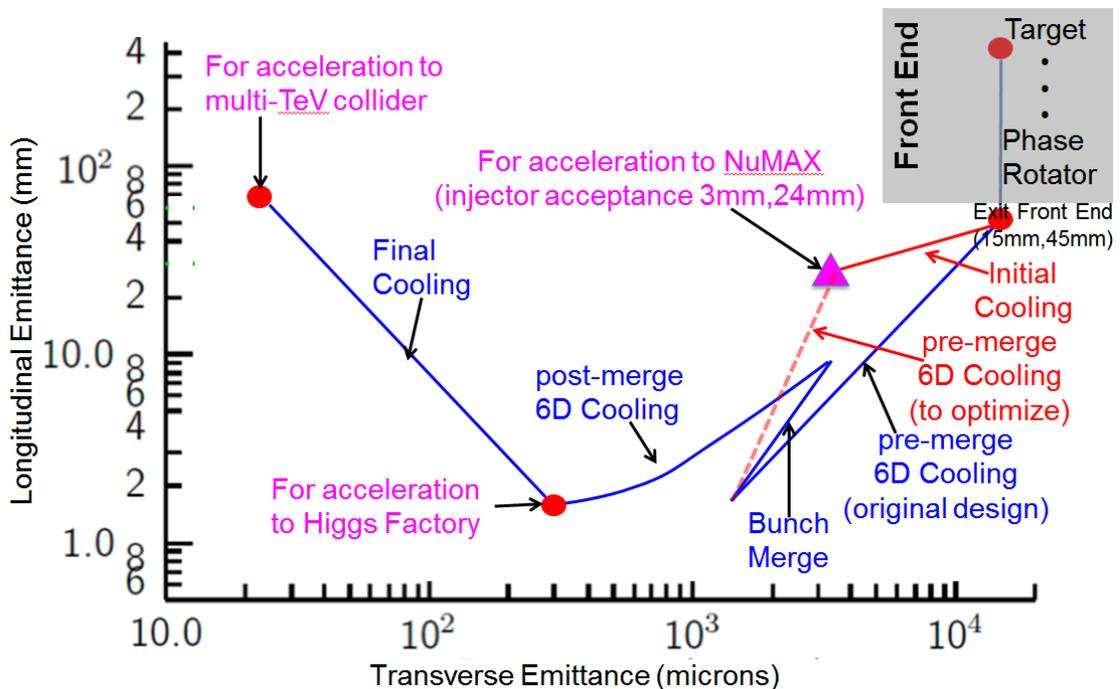
Figure 2: 6D cooling path to be re-optimized with initial cooling
