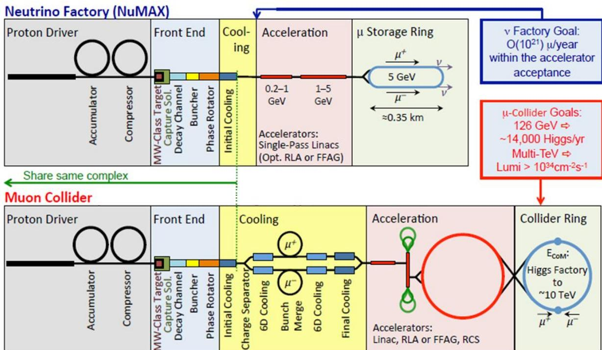
Figure 1: Neutrino Factory and Muon Collider layouts emphasizing synergies
