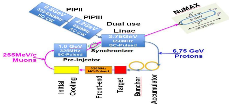
a) Layout of a Muon based Neutrino factory
