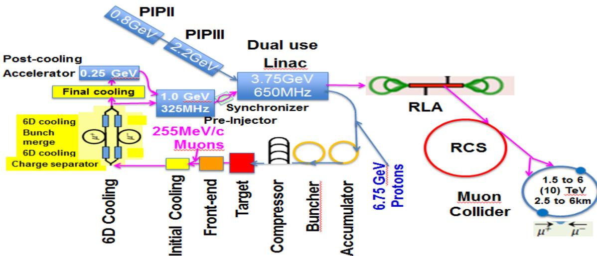
c) Layout of a multi-TeV Muon Collider
