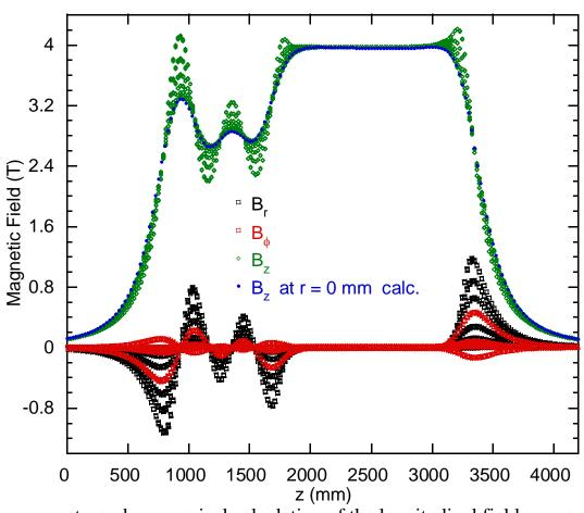
Measured field components, and a numerical calculation of the longitudinal field on magnetic axis using "as-built" coil parameters.
