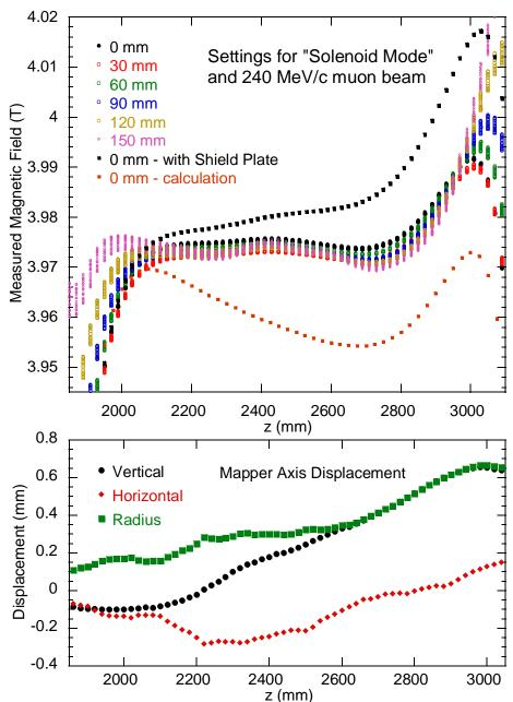
B<sub>z</sub> magnetic field component in the tracker region: measurements for 3D Hall probes at different radii for a case without shielding plate, measurements at 0 mm for a case with shielding plate, and a numerical calculation on axis (no shielding plate) using "as-built" coil parameters and measured coil currents.
