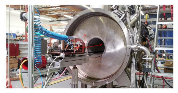
X axis along the magnet on direction: SSU opposite to beam direction; SSD in direction of the beam Z axis vertical
