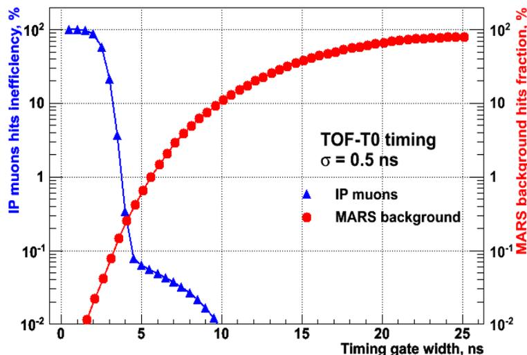
Inefficiency of IP muon hits and surviving fraction of MARS background particle hits in the VXD and Tracker Si Detectors versus width of timing gate for hit time resolution of 0.5 ns
