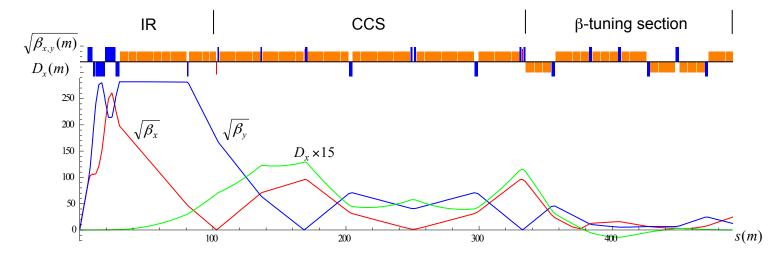
Preliminary version of the 3TeV collider lattice with quadruplet Final Focus.  $\beta_y^{(max)}$  is reduced to 80km compared to 118km in the previous design with triplet FF. Matching to the arc has not been done yet.
