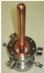
Power coupler, the antenna feeding up to 300 kW RF power to the cavities.
