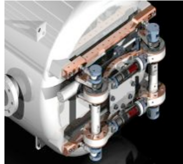
Cold tuner, to mechanically fine-tune the 352 MHz resonance frequency.
