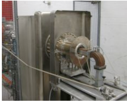
Prototype proton source operational, and under further development, in Catania. Output energy 75 keV.
