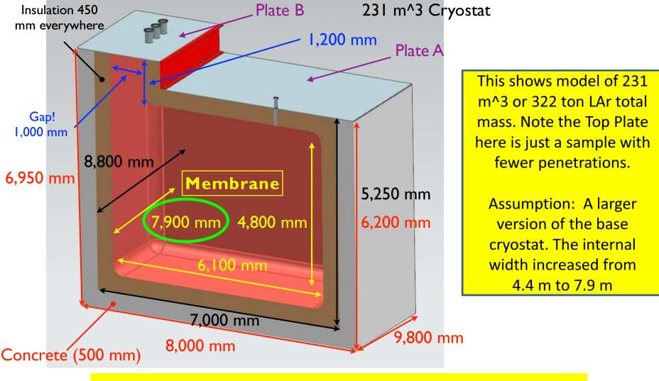
• This is the 3D model of LAr1-ND based on the 35 ton concept.
