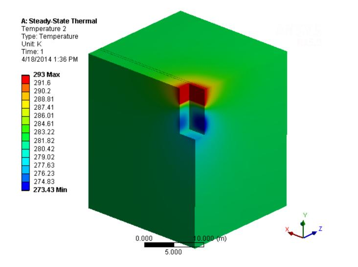
With 400W Floor Heater and 200W Large Side Heaters (800W Total) the concrete along the sides reaches a minimum temperature of ~273K. If the structure if free standing and is does not lay against the soil, the temperatures will be even higher.
