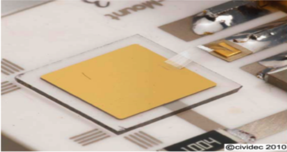
Figure 66. Diamond-based secondary emission monitor
