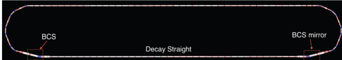
Figure 31. Racetrack ring layout. Pions are injected into the ring at the Beam Combination Section (BCS). Similarly, extraction of pions and muons at the end of the production straight is done using a mirror image of the BCS.
