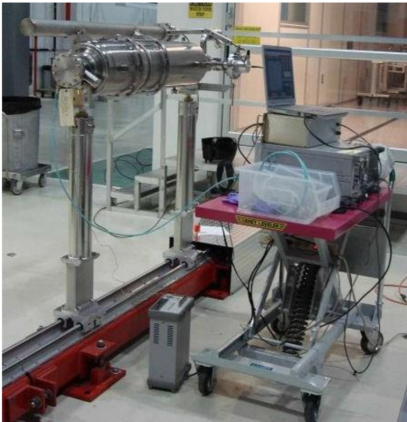
Figure 45. Typical Set-Up of Dressed SRF Cavity for Pressure Test.
