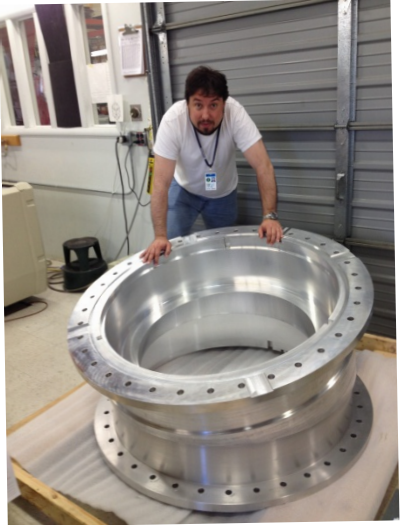
Machined shell ready for inspection
