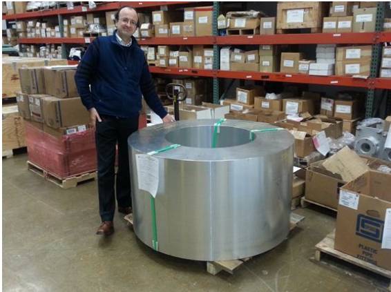
Outer support cylinder casting pre-machined
