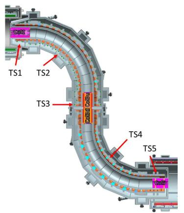
There are four collimator elements. COL3u and COL3d are located in TS3 and they are used to filter particles based on electric charge and momentum.
