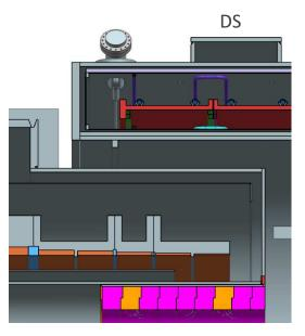
There is a physical overlap of around 940 mm between the DS and TS cryostats. When the TS is at full power, there is a net axial force of around 100 Tons pulling the TS and the DS together.
