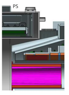
Due to space constraints, the primary proton beam pipe must be routed through the TS cryostat. When the TS is at full power, there is a net axial force of around 130 Tons pulling the TS and PS together.
