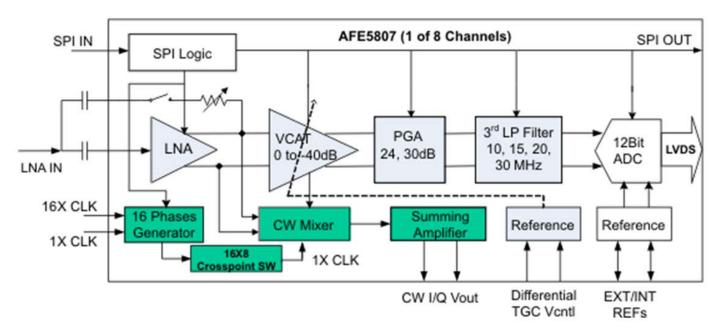
Eight channels of: low noise preamp, variable gain amp, programmable gain amp, programmable low pass filter, 80msps 12 bit ADC. \$8 per channel, 120mW per channel. Adjust gain such that 1p.e. = 10 ADC counts.
