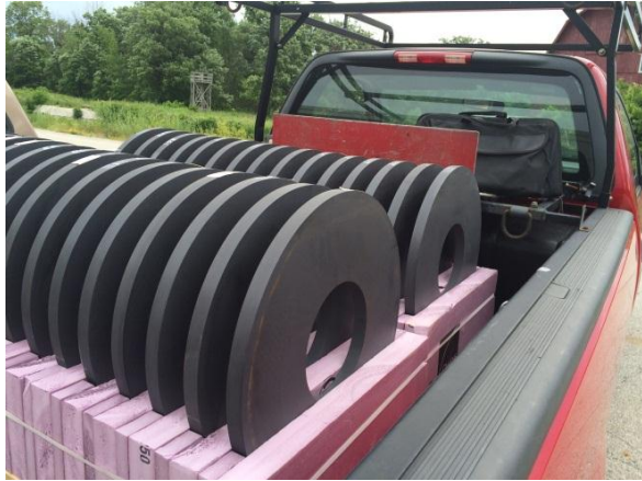
Figure 7: In this image are several of the ferrite cores harvested from decommissioned cavities.
