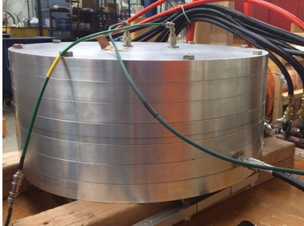
Figure 4: Five ferrite test fixture. The RF input can be seen in the lower right side of the image.
