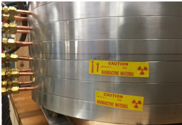
Figure 5: Reverse side of the test fixture. The copper water tubing can be seen on the left of the image.
