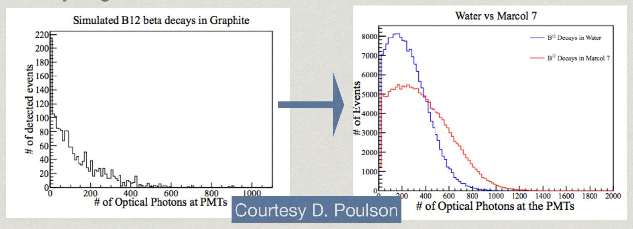
Solution: Replace water with mineral oil to produce <sup>12</sup>B in the ID volume
