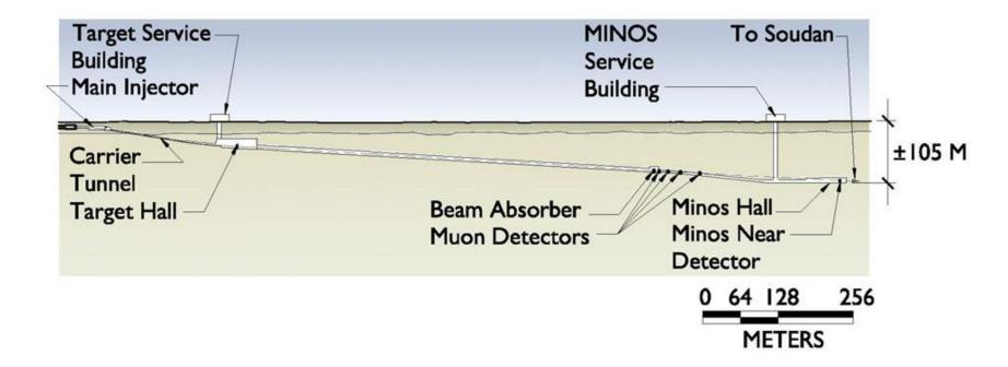
For NuMI we have a deep beam facility mined in underlying rock strata with the design driven by length of the decay pipe (675 meters). Initially we started with a similar design for LBNE.
