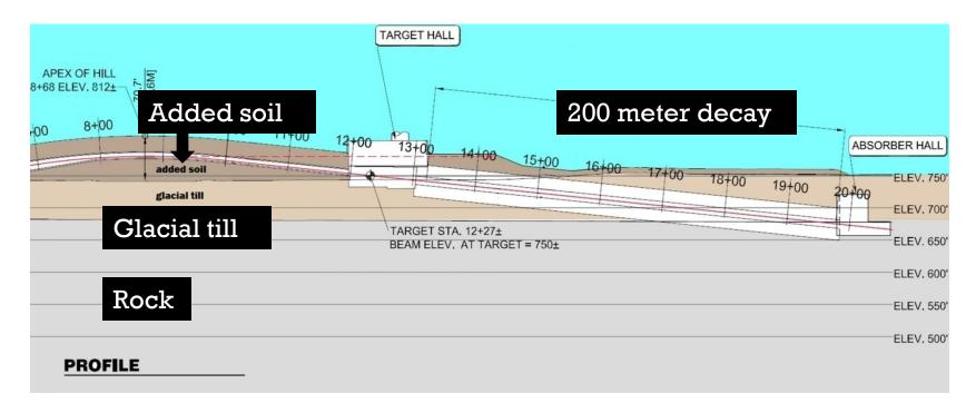
Much shorter decay than NuMI (now ~ 200 m) enables target hall elevation placement out of under-lyimg rock. Design is chosen to balance construction requirements for elevated proton beam versus decay region and absorber located partially in rock. Advantages of significantly reduced cost [ > \$ 125 million savings] and improved tritium mitigation compared to a NuMI style deep beam design for LBNE.
