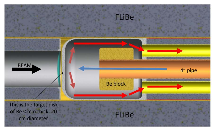
All the metal inside the Li/FLiBe is beryllium to allow neutrons to get into the FLiBe. Arrows indicate water flow.
