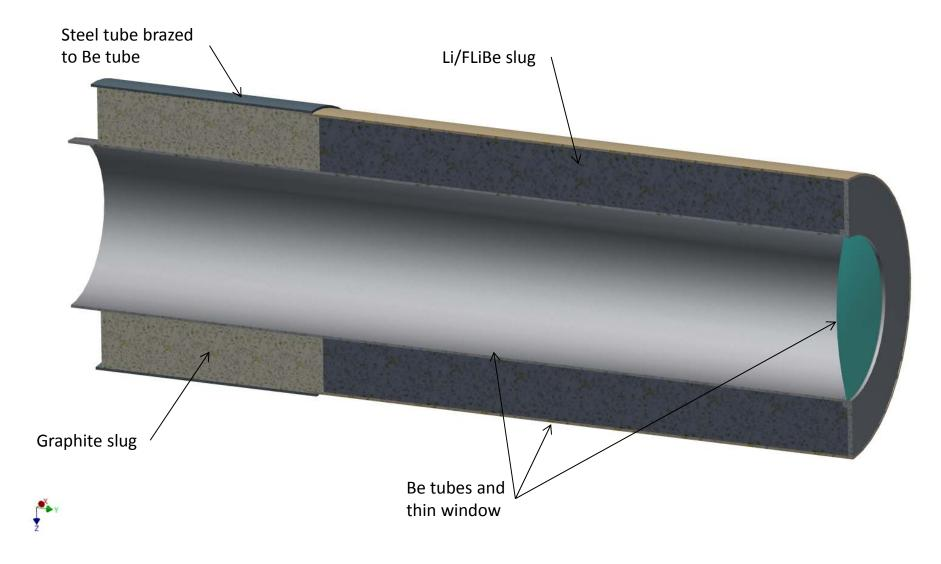
We need to look at the energy deposition in the thin window and check whether air activation will be an issue. This work is in progress.
