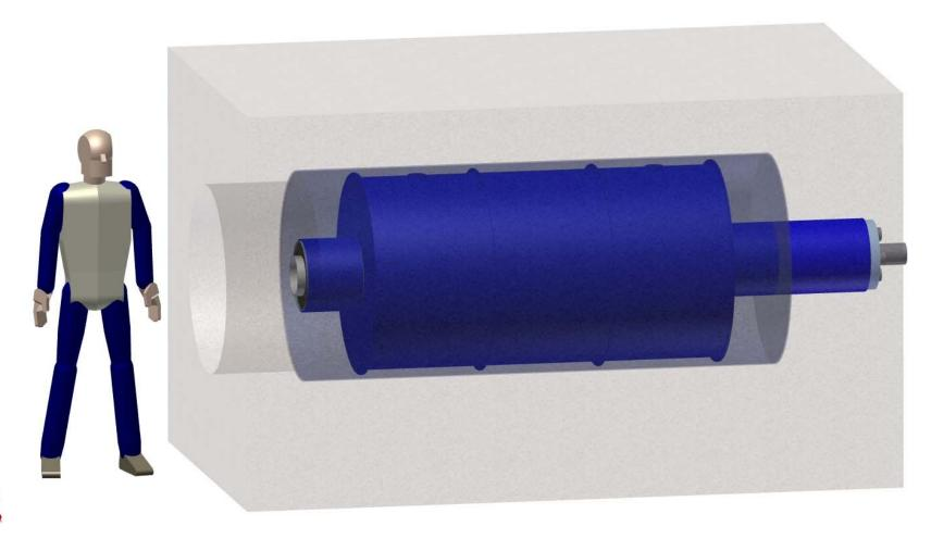
At this point, FLiBe looks more benign than elemental Lithium. Either one can be cast inside this tank, but to cast the lithium the whole thing has to be done in an inert atmosphere making it much more complicated.
