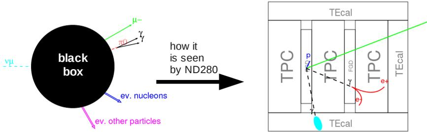
**FIGURE 2.** Inclusive  $\nu_\mu$ CC $\pi^0$  reaction definition and its manifestation in the ND280 detector
