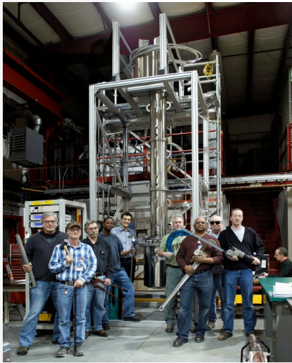
Distillation column to produce ^{39}\text{Ar} depleted Argon for dark matter community, such as Dark-Side
