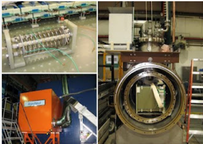
ArgoNeut TPC field cage and installation in NUMI underground lab.
