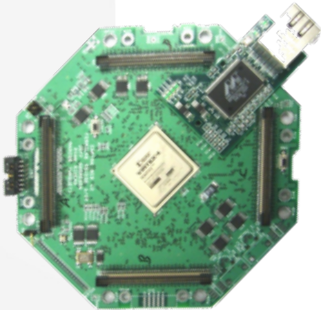
“Green Board” NPCB – Node Processing and Control Board
