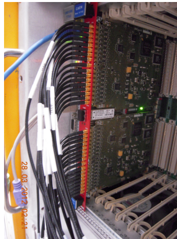
CAEN 1742 module digitizes at 5 Gs/s. Good for timing and energy measurement
