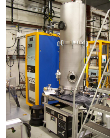
Thin film coating plant for 8" plates
