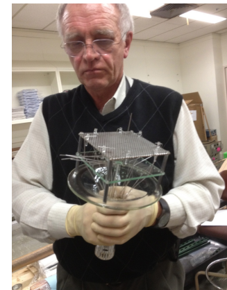
Anatoly Ronzhin holding the 'chalice' for systematic photocathode testing
