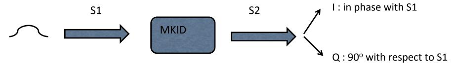
Q & I measured relative to S1 S<sub>21</sub> is the sum in quadrature of Q & I
