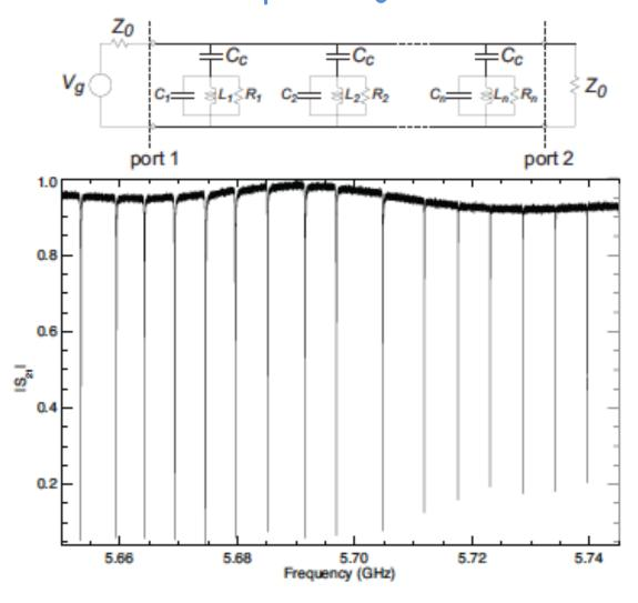
Large array of superconducting detectors are NOW possible.
