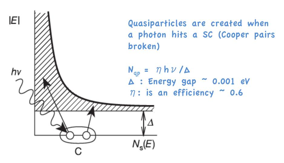
Number of quasiparticles is proportional to photon energy! ~5000 quasiparticles for a visible photon
