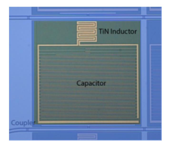
Light is collected at the inductor (micro-lens needed for fill factor)
