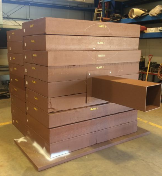
Assembled M4 Diagnostic Absorber waiting to be installed on the tunnel GPP.
