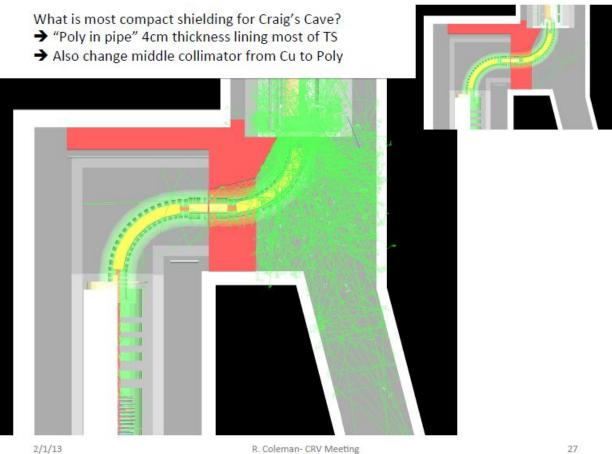
Red material is a mixture of stainless steel and borated poly
